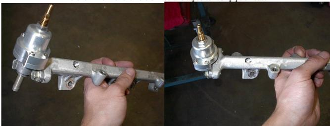
Well here is my first attempt at mounting the gauge, yes it worked but there is a big problem with doing it this way. Being extended so far out when I revved the engine the gauge and most of the extension pipe would vibrate back and forth like crazy! No good, either it will slowly loosen itself causing an inconvienient leak or it will simply weaken over time and crack in half possibly causing a fire and stranding me.
