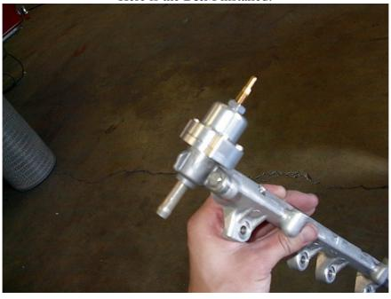
Now for the gauge install. The gauge I got has a male 1/8" pipe thread on it and I didnt see any place before the rail I wanted to try and adapt it to.
