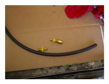
Wrap a ton of the teflon tape around the fitting thread and screw it in nice and tight. (They like to leak.) Then force the hose on. Yes you will have to push really hard to get it on, this is normal, make sure it seats against the plastic base on the fitting. Now though it's not technically required I backed that up with a small hose clamp, dont over tighten it though.
