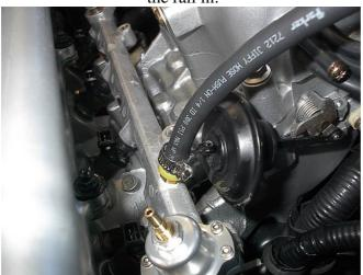
Now figure where you want to mount the gauge and how you want to route the hose. Once the hose is cut to the length you want force the fitting on the end, teflon tape all the threads and tighten everything up. When you first start the car before doing anything else watch for fuel leaks, keep an eye on the fitting, hose, and where the injectors slip into the rail.
