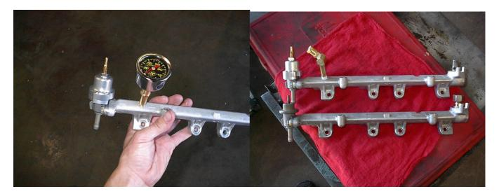
The solution! I picked up some "Lock-On" barb fittings and 2ft of 300psi rated hose (Make sure the hose is fuel compatable!) Also make sure the fittings arent just regular barb fittings you can tell the diffrence because the lock-on ones have that little yellow plastic ring that the hose end will seat against.
