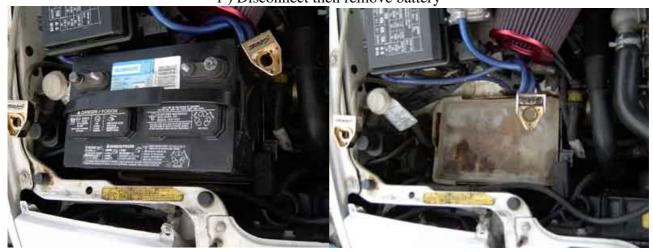
2 ) Remove tray and mounting bracket (bracket is pictured to the right of the battery perch). Use a 10 mm socket
