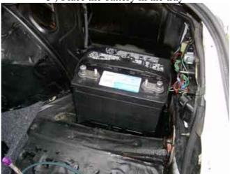
6) Secure and Wire up the battery. Make sure the ground wire is as short as possible and secure - otherwise this could cause some power problems and potential noise interferance through the stereo
