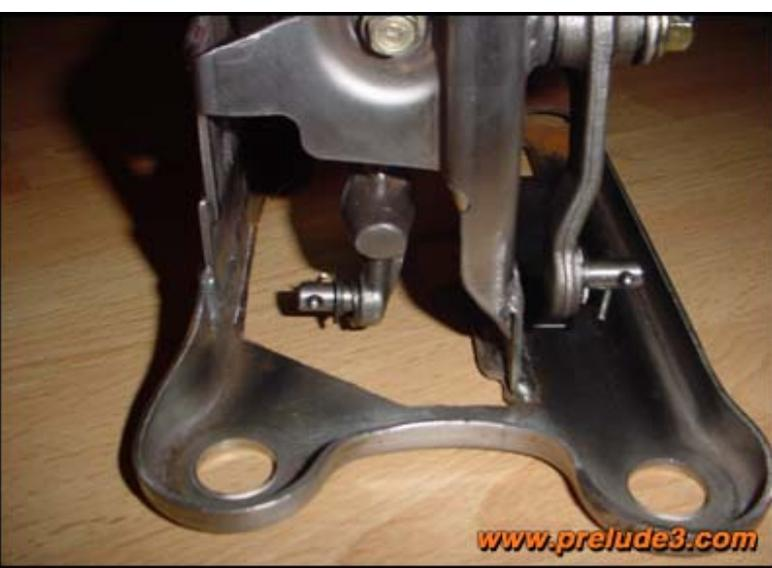
Clearly visible here is the hammer-like thingy located on the shift lever. It ensures that the lever cannot be pushed forward or backward too far, so that the ball joint operating the lever in the bracket isn't stressed too much.
