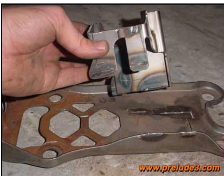
After cutting all welds, the bracket is detached from the frame.
