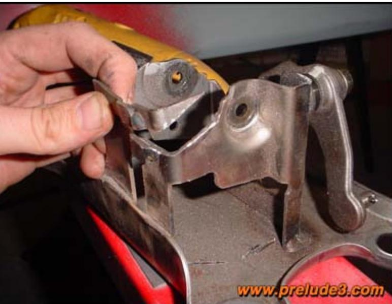
Because the bottom of the lever will be extended, the bracket that holds it has to be raised. I ground some material off the top of the bracket, so that the plastic center console barely fits over it.
