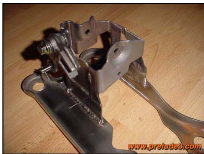
This is the modified shift lever. The top is rethreaded and the bottom is extended by 2.5 centimeters, by welding in between a piece of the cut-off top.
