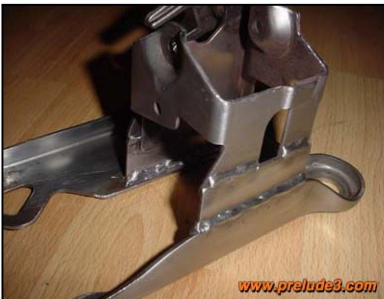
The bracket is raised two centimeters by welding in two metal plates on both sides.
