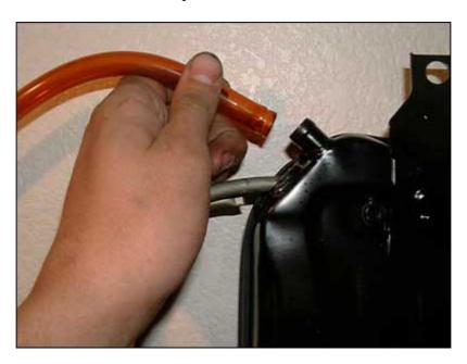
The solution is easy. Simply pull the drain tubes out of the drain holes and clean the end of the tubes where the clogging generally occurs. There are drain tubes that run through all four roof pillars of the car. However, the rear two pillars tend to clog the most.
