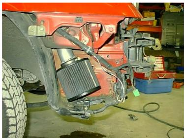
Now just put the bumper cover back on and mount the coolant reservoir if you want to and you are done. Another thing about this mod is that the sounds coming from the filter bounce of the ground and sound very loud. Even the air being sucked into the filter on a non-turbo car sounds good.
