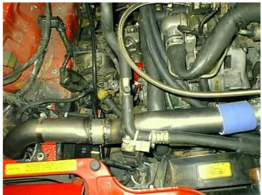
The next pic is a shot of the filter in its new home. It is mounted to the intake pipe.
