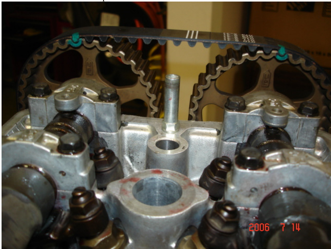
This pic shows the belt with the tension set.
