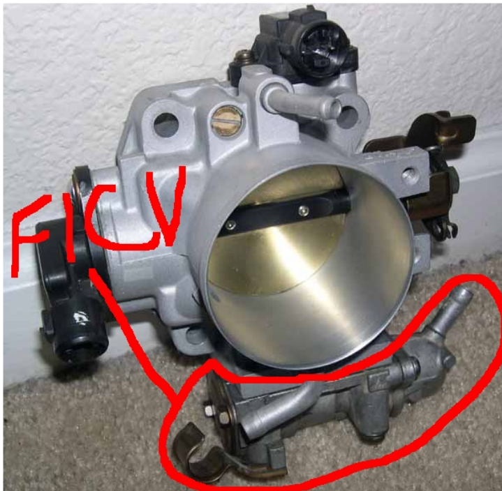
Picture of other b-series with the FICV on throttle body:
